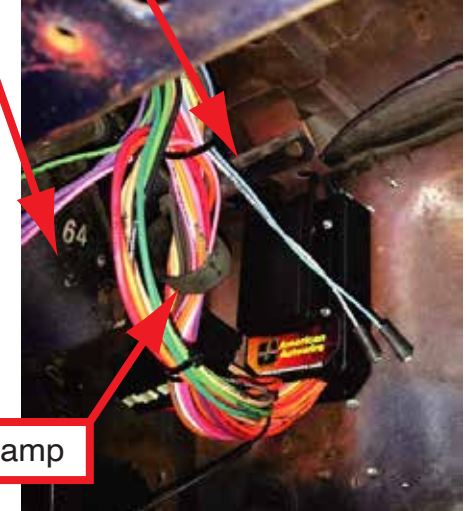
Harness routed through loop clamp
